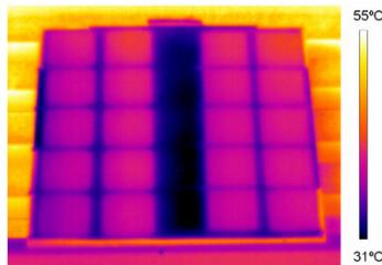
**Figure 5:** IR imaging of monofacial (left) and bifacial (right) modules showing no significant difference in the operating temperature.
