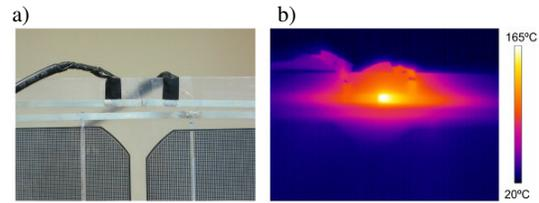
**Figure 3:** Visual and infrared images of in-laminate bypass diode, after forcing a current of 10 A through the diode for a period of 1 hour.
