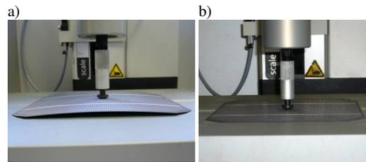
**Figure 2:** 110 $\mu\text{m}$  thick solar cells interconnected a) by SnPbAg soldering and b) with conductive adhesive.
