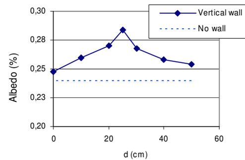
**Figure 6:** Example of albedo optimization by including a white vertical wall behind the module at varying distances. It is observed that for 25cm distance the albedo is increased by 20% with respect to the system with only a white ground and no vertical wall.
