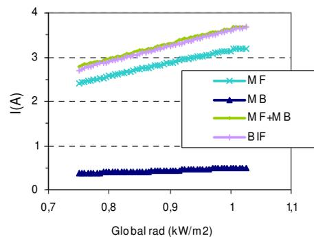
**Figure 1:** Short-circuit current of a bifacial module measured by covering the back-side (MF), covering the front-side (MB) and in bifacial configuration (BIF). The measured data show the linearity of the short-circuit current.
