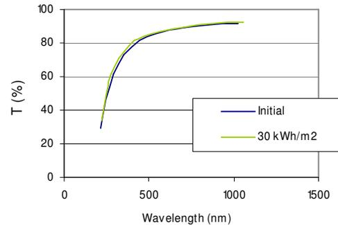
**Figure 4:** Transmission of ETFE backsheets before and after receiving 30kWh/m<sup>2</sup> of UV radiation. The variations are within the measurement tolerances.
